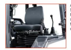
Adjustable Suspension seat Provided as standard feature for enhanced operator comfort.
