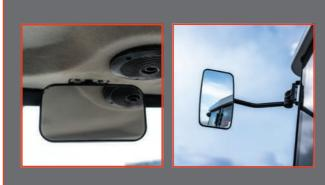
Large Side view mirrors and additional rear view mirror improves rear visibility for more convenient and safe operation.
